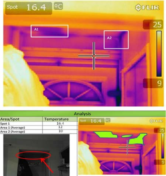
Figure 6: Using thermography for the entrance
