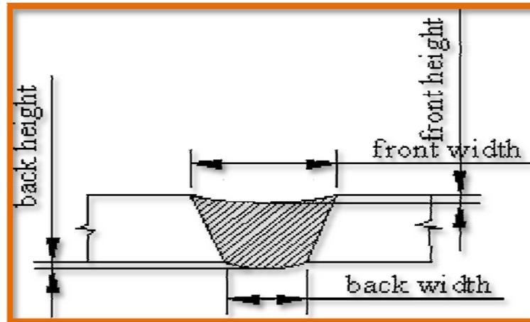
**Figure 1:** Typical weld pool geometry.
