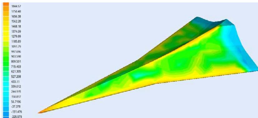
**Figure 1:** Distribution of heat flows on the surface of the winged vehicle at  $M_\infty = 17$ . Non-catalytic surface. In a yellow - temperature of 1278 K.
