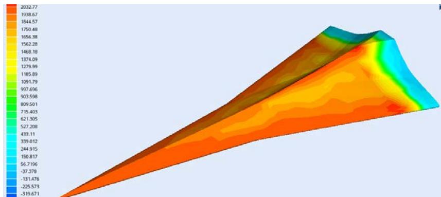
**Figure 2:** Distribution of heat flows on the surface of the winged vehicle at  $M_\infty = 17$ .
