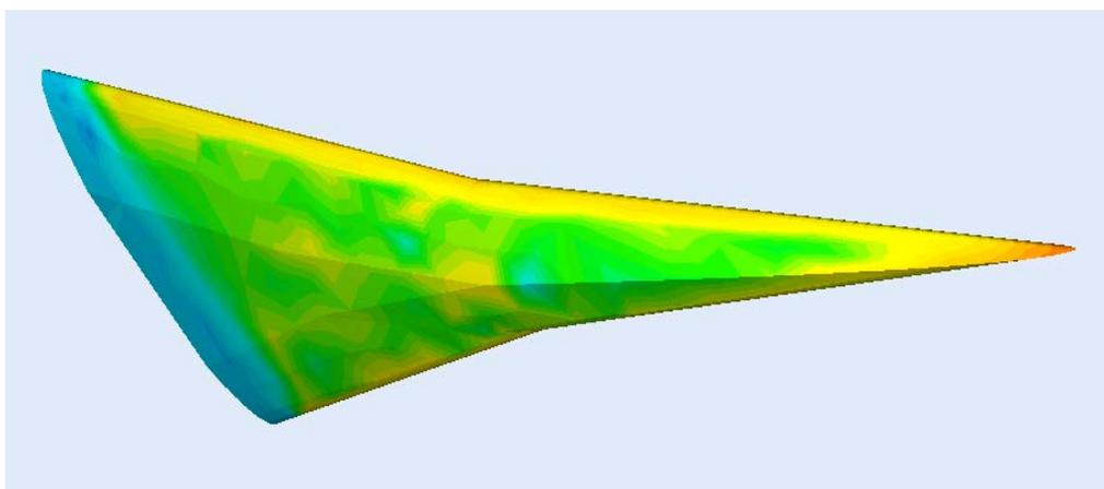
**Figure 3:** Distribution of heat flows on the surface of the winged vehicle at  $M_\infty = 17$ .
