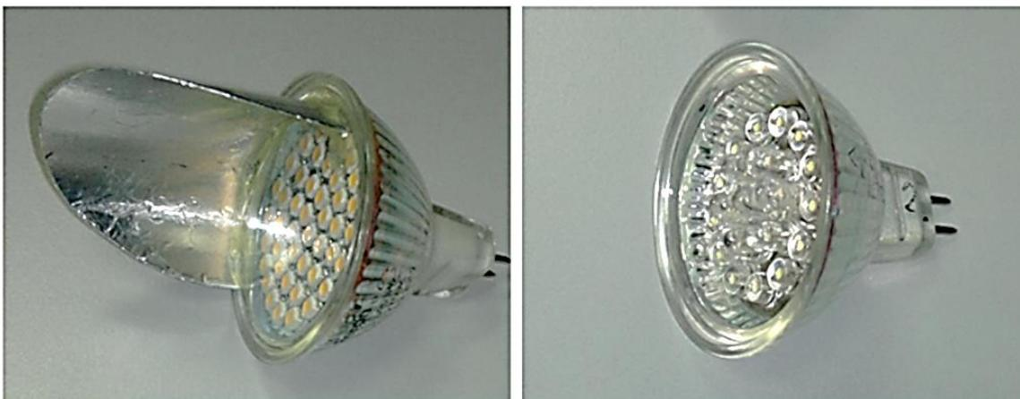
**Figure 2:** Light sources used in the photometric experiment: 1 - kososvet, 2 - LED lamp
