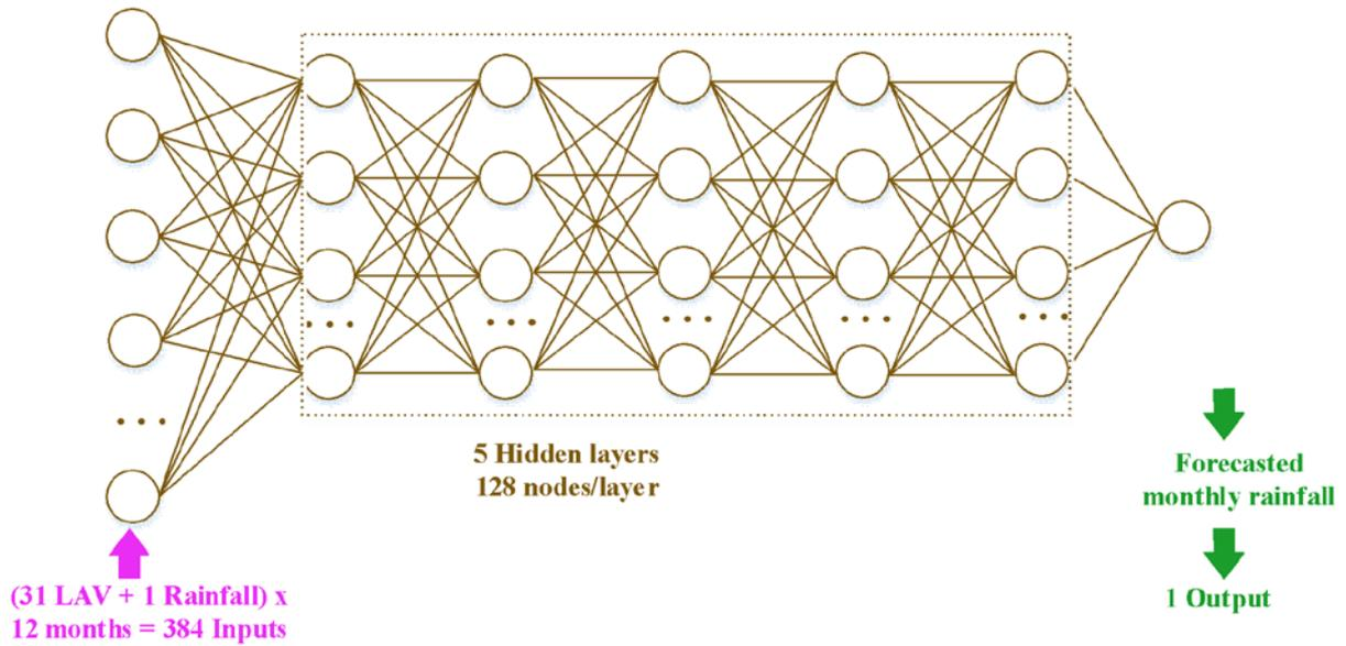
**Figure 2:** DNN architecture developed with 384 inputs to predict the monthly rainfall forecast.
