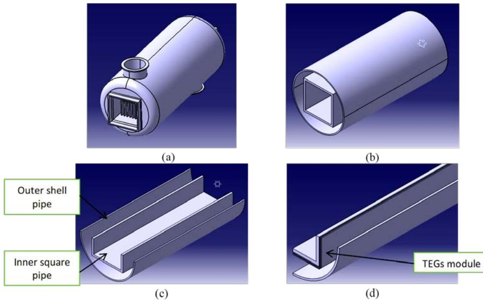
**Figure 1:** CAD drawing for the heat exchanger, (a) The initial detailed drawing geometry before simplified for the analysis; (b) The simplified drawing geometry for the analysis consists of the outer shell pipe and the inner square pipe only; (c) The simplified drawing geometry is cut into half as the geometry is symmetry; (d) TEGs attached to the pipe assembly
