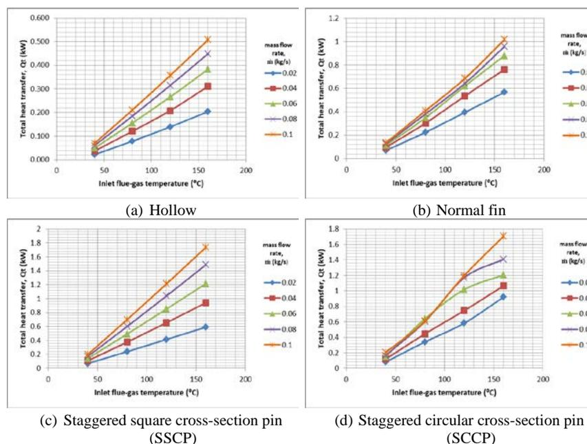
**Figure 2:** The graph shows the total heat transfer ( $\dot{Q}_t$ ) versus inlet flue-gas temperature ( $T_{h,in}$ ) for each heat exchanger design with different flue-gas mass flow rates.
