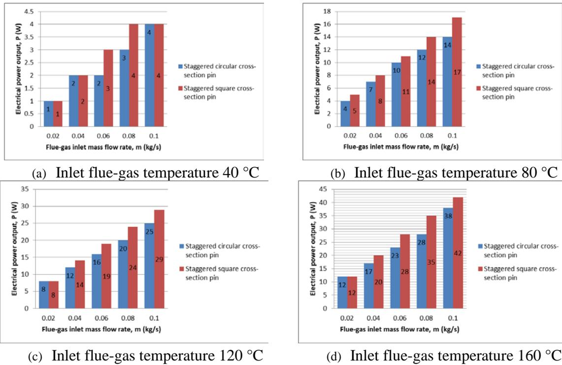
**Figure 5:** The electrical power output ( $P$ ) versus the flue-gas inlet mass flow rate ( $\dot{m}$ ) for both heat exchanger geometry at each inlet flue-gas temperature.
