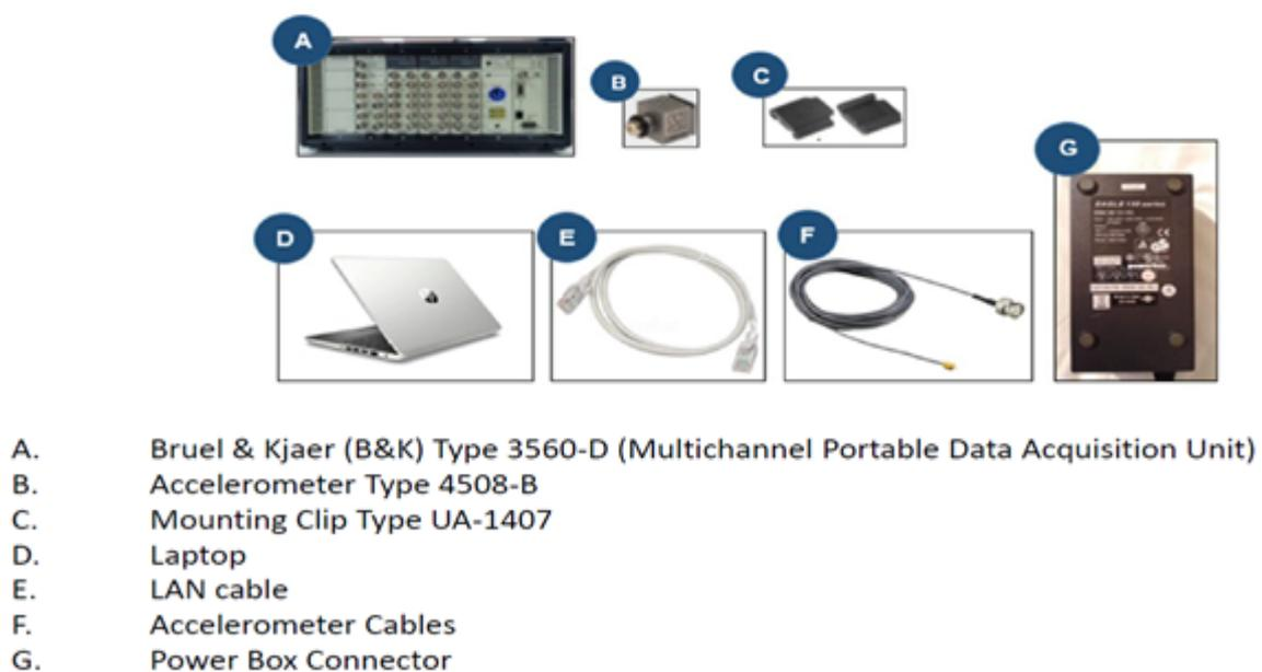
**Figure 1:** Bruel & Kjaer PULSE™ Multi-Analyzer System connect to a computer with MTC™ and OMA Pro™ software.
