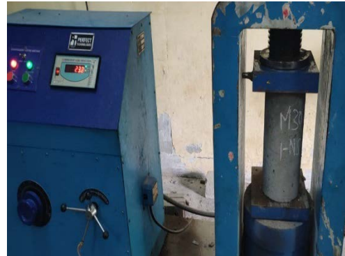
Figure 6: Cylinders Compressive Strength Test
