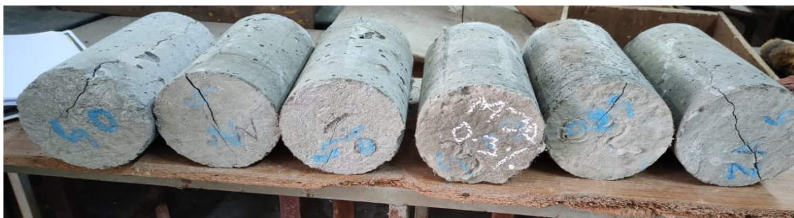
Figure 14: Failure Pattern of Cylinder Specimens
